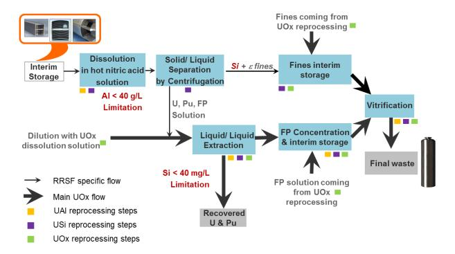
Fig 5. UAI and Silicide RRSF reprocessing at La Hague, process diagram
