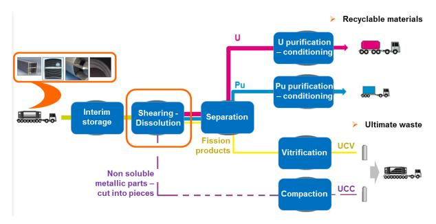
Fig 4. Process diagram for RRSF reprocessing on La Hague site
